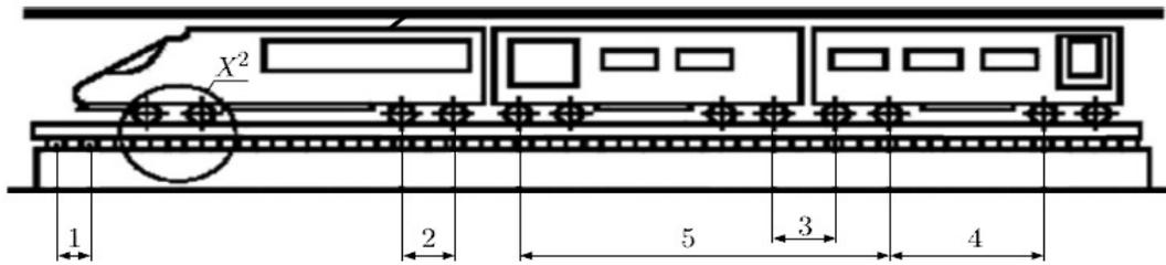
Fig. 1. **Characteristic parameters of vibration source:** 1 – distance between supporting elements of the track; 2 – distance between wheelsets of the bogie carriage; 3 – distance between the adjacent bogie carriages of the adjacent railcars; 4 – distance between bogie carriages of one railcar; 5 – distance between railcars
