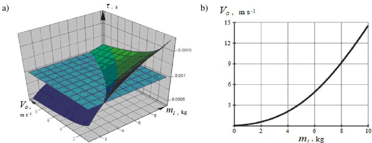
Fig. 5. Result of construction of three-dimensional surface of impact function  $\tau = F(m_1, \vartheta_0)$ , at  $R = 0.05$  m,  $E_1 = 1.8 \cdot 10^6$  N·m<sup>-2</sup>: three-dimensional function surface and plane  $\tau = 0.001$  s (a), intersection curve of three-dimensional surface and plane  $\tau = 0.001$  s (b)
