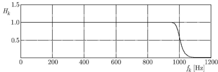
Fig. 4. Butterworth filter characteristics in low frequencies domain at  $f_H = 0.1$  Hz,  $f_B = 1000$  Hz,  $p = 50$
