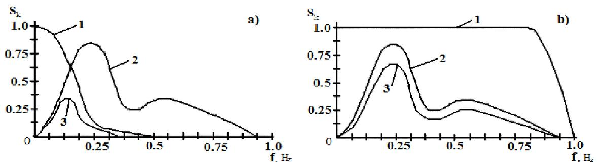
Fig. 3. Dependence response spectrum of system on frequency response characteristics with a shock duration greater than the optimal (a), optimal duration of the shock-impulse (b): 1 – spectrum of impact on the system; 2 – own spectrum of the system; 3 – spectrum of the response system to impact
