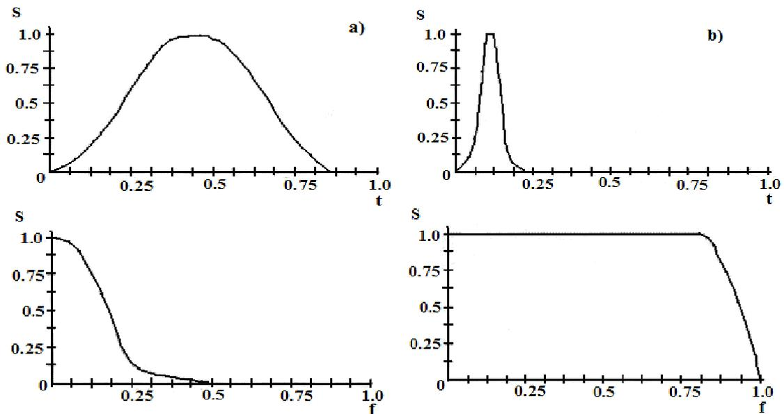
Fig. 2. Dependence of frequency spectrum impact on duration of shock-impulse: when the shock duration is longer than the optimal one (a), at the optimum duration of the shock-impulse (b)
